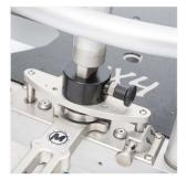
Steering system: The steering system of the 4×4 Dolly is made of special, very hard steel. It ensures the durability of the switchgear unit.
