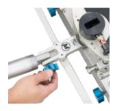
Alternative steering mode: The steering rod can also be used as drawbar, e.g. to better handle a crane mounted on the dolly. 3
