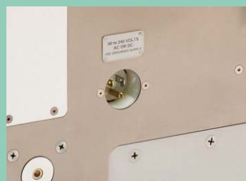
Power Requirements: 90 TO 240 VOLTS AC OR DC
